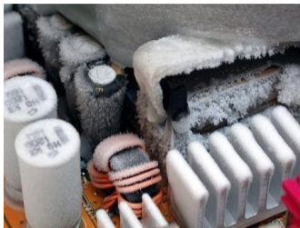
Liquid nitrogen for CPU overclocking
